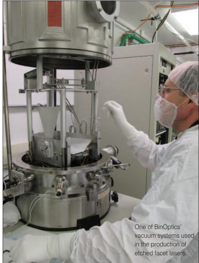
One of BinOptics' vacuum systems used in the production of etched facet lasers.
