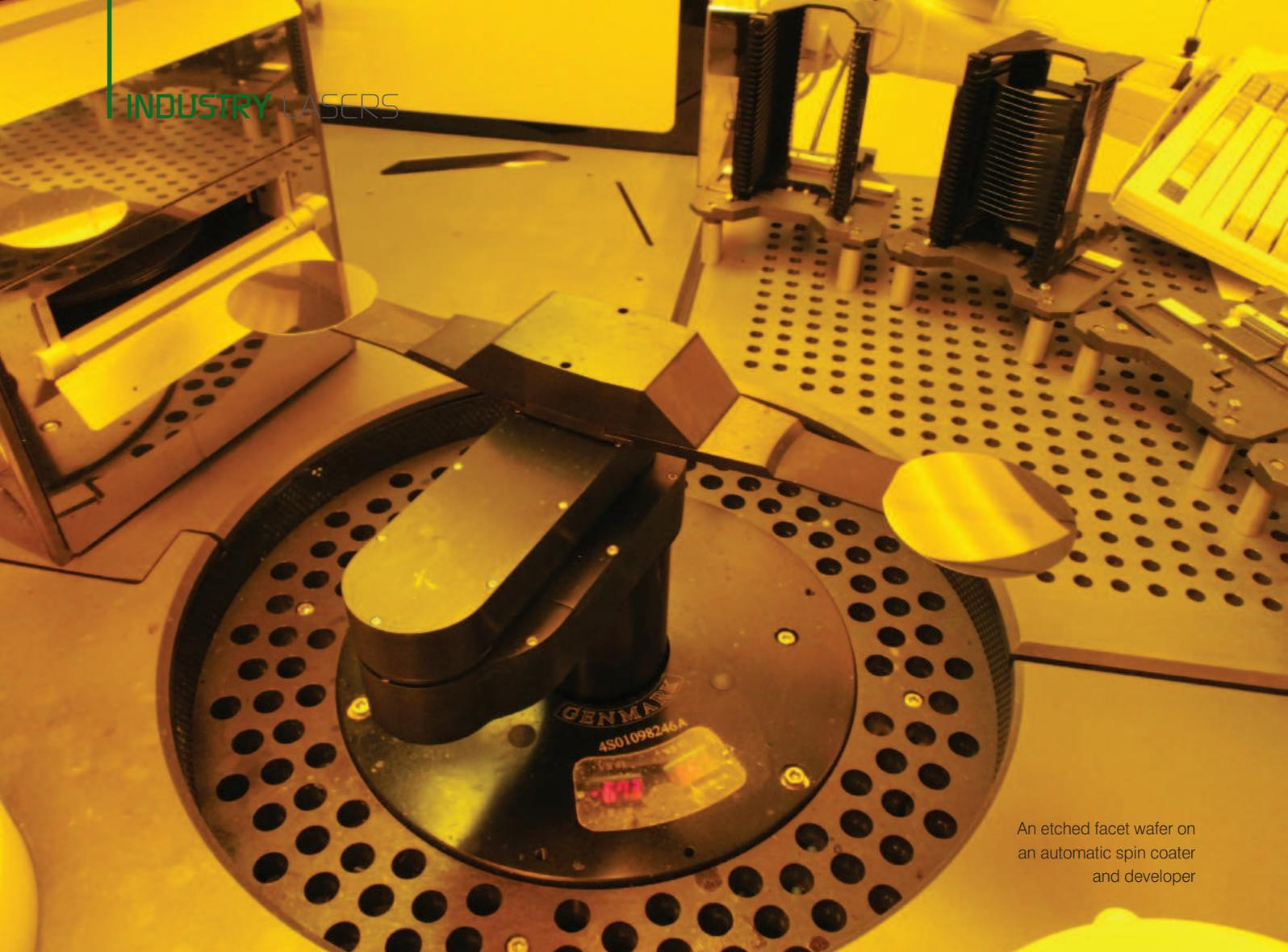
An etched facet wafer on an automatic spin coater and developer
