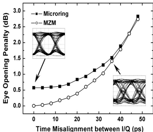
Fig. 3. EOP as a function of time misalignment between  $I/Q$  data streams.
