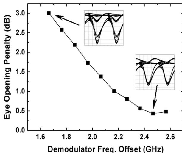
Fig. 4. EOP of using the microring-based demodulator drops with demodulator frequency offset.
