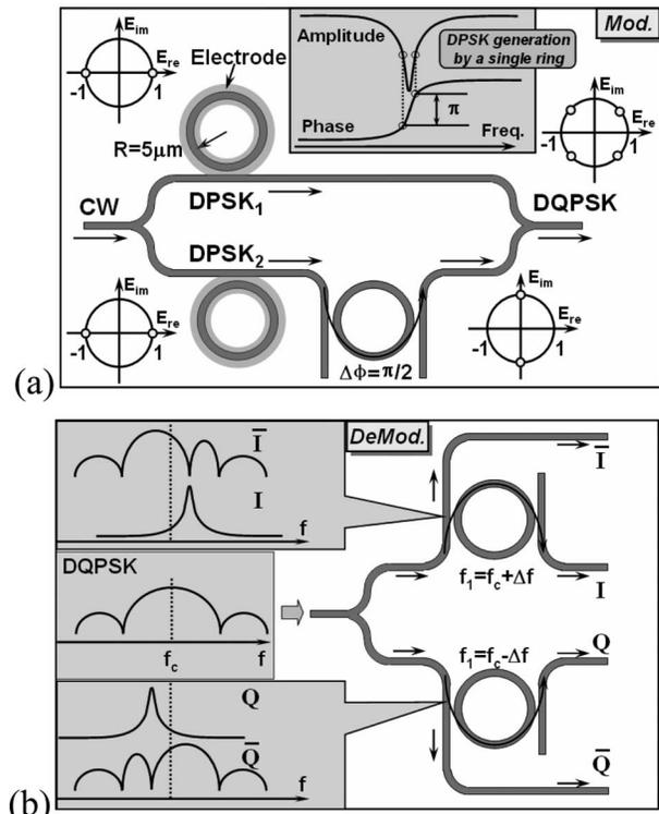
Fig. 1. Microring-based DQPSK (a) modulator and (b) demodulator.
