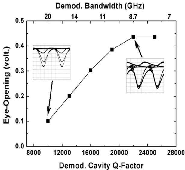
Fig. 5. EOP is improved with a demodulator bandwidth of 8.7 GHz.
