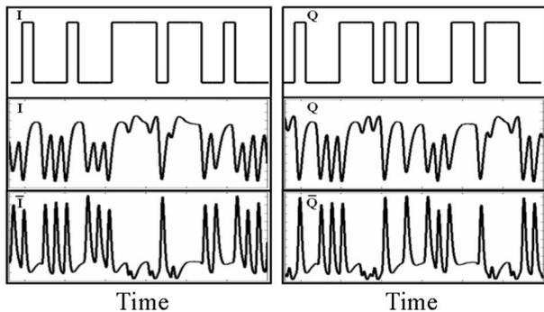
Fig. 6. Original logic pattern, demodulated  $I/Q$  data, and their inverted versions.
