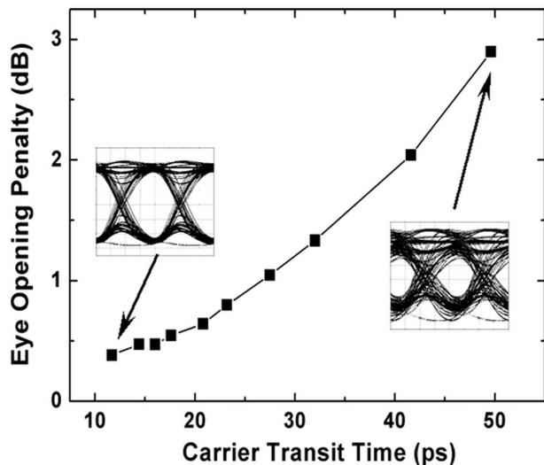
Fig. 2. EOP of the DQPSK signal increases with transit time from 12 to 50 ps.
