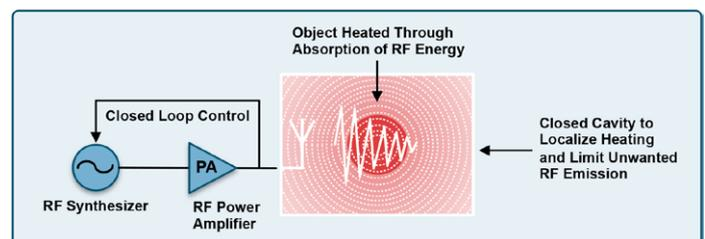
Figure 1 Solid-state powered RF energy application
