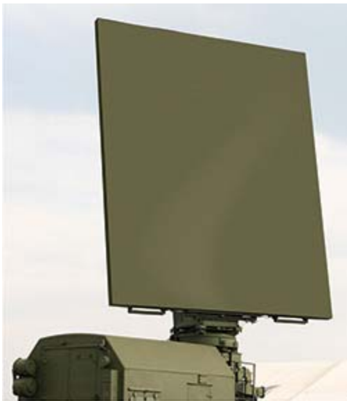
Figure 1 The active phased array architecture enables the beam to be electronically steered and multiple radars to be combined in a single system.
