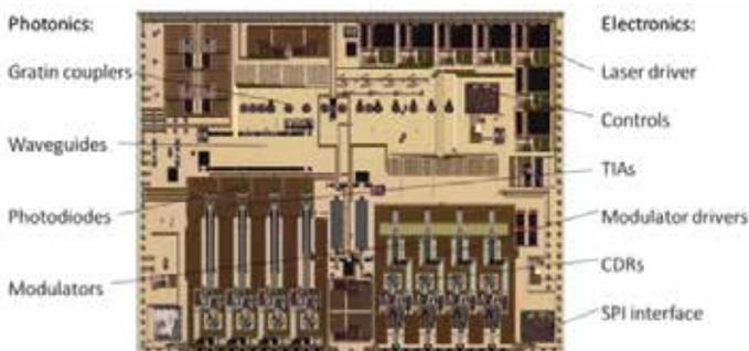
Sicoya’s monolithically integrated 100G electro-photonics IC (Image: Sicoya)
