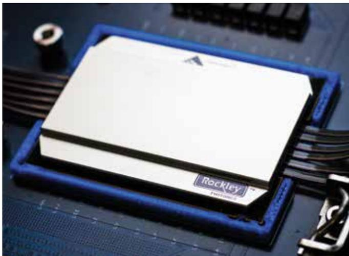
Rockley Photonics showed its Topanga 12-port 100G Ethernet switch at OFC ’18. (Image: Rockley Photonics)
