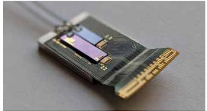
Transmit-receive optical subassembly (TROSA) for data communications using Rockley Photonics’ silicon photonics platform (Image: Rockley Photonics)
