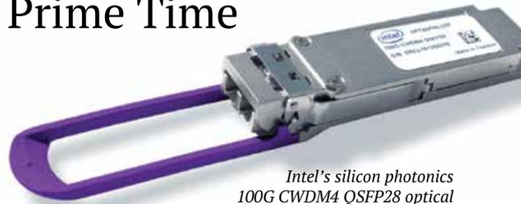
*Intel's silicon photonics 100G CWDM4 QSFP28 optical transceiver supports extended-temperature-range operation. (Image: Intel)*
